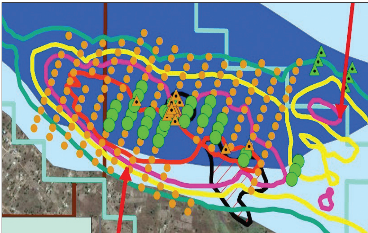
Figure 8. The above historical prospecting on Kashitu highlights: a) BHP RAB drilling – orange dots, b) BHP RC drilling – green dots, c) historic diamond drilling – orange triangles, d) Zn-in-Soil anomalism – red outline > 15 000 ppm Zn, and, old workings – black outline. Current objective includes defining an area of near-surface anomalism within the target area highlighted by the soil-geochemistry
