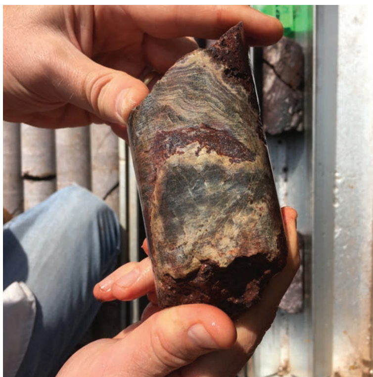
Very coarse grained massive/semi-massive willemite with hematite (specularite) and calcite
