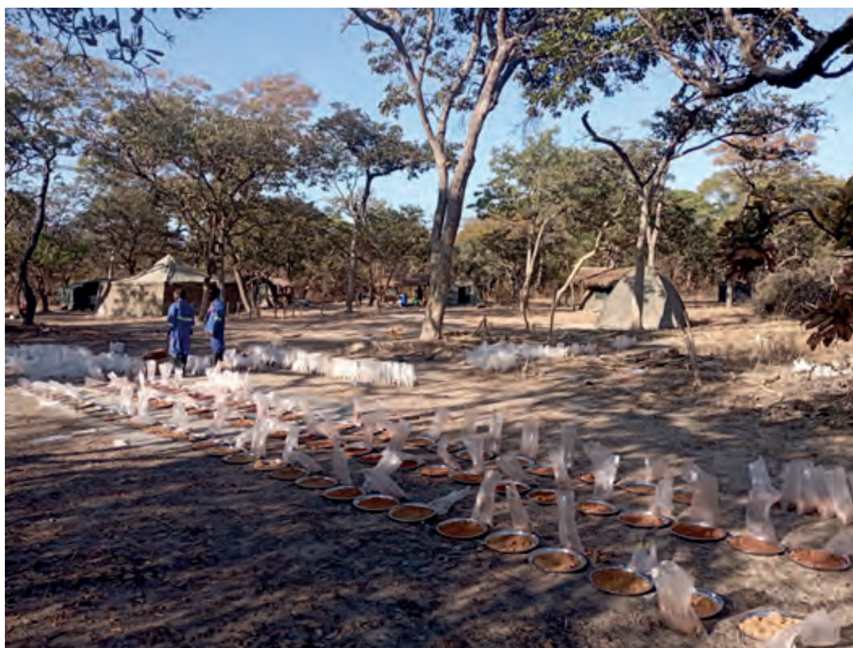
Photo 4: Drying and sorting soil samples at Shinganda in preparation for pXRF analysis
