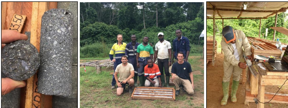
Figure 6: Disseminated galena (Pb) and sphalerite (Zn) mineralisation encountered in DKDD078 (33.5m) at Dikaki – assays pending (LHS); and the site team at work within the Dikaki Prospect (RHS).
