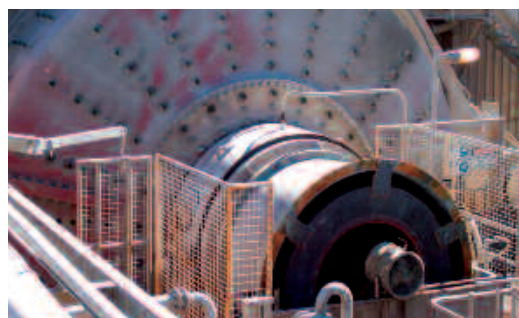
A SAG mill in situ, similar to one being refurbished for the Philippines gold mine.
