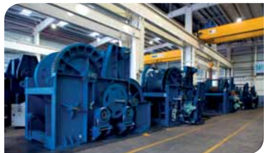
Anchor Handling Winches Being Assembled
