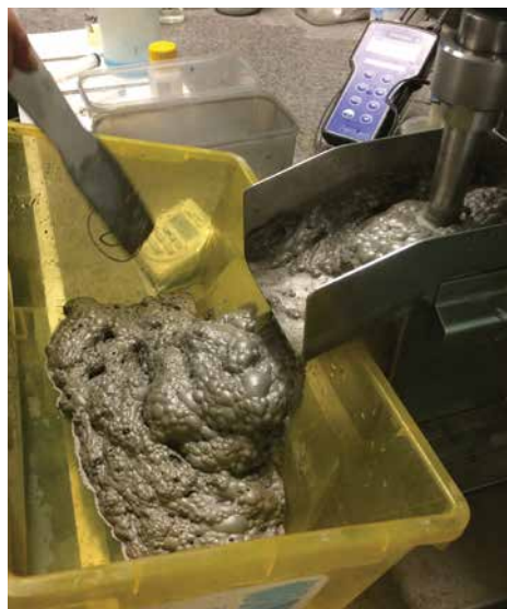
Figure 2a - High grade (54-59%) zinc concentrate produced by the 2nd cleaner stage of test AF8.
