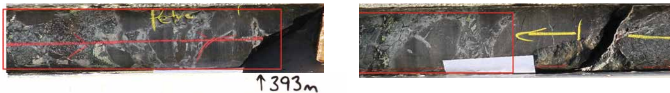
Figure 8 - Photo of Netley ALN001 drillcore from 392.8 to 393.0 and 393.6 to 393.8 metres with intersected copper (chalcopyrite) highlighted.
