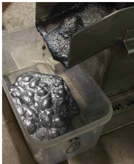
Figure 2b - High grade (47-64%) lead concentrate produced by the 2nd cleaner stage of test AF8.
