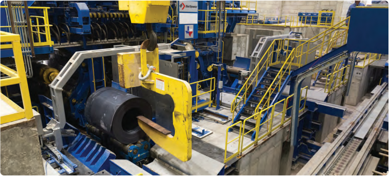
Sinton Steel Mill hot rolled coil coming off the coiler at the hot strip mill.
