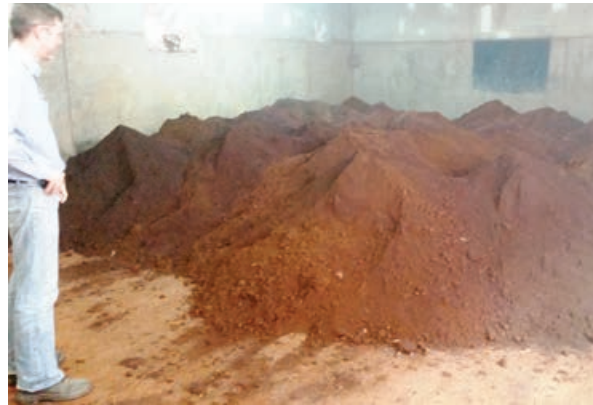
66 tonne sample of weathered typical mineralisation in Perth being prepared as feed for the pilot plants.
