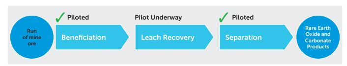
Three stage process developed by Peak for Ngualla's rare earth mineralisation and pilot plant status.
