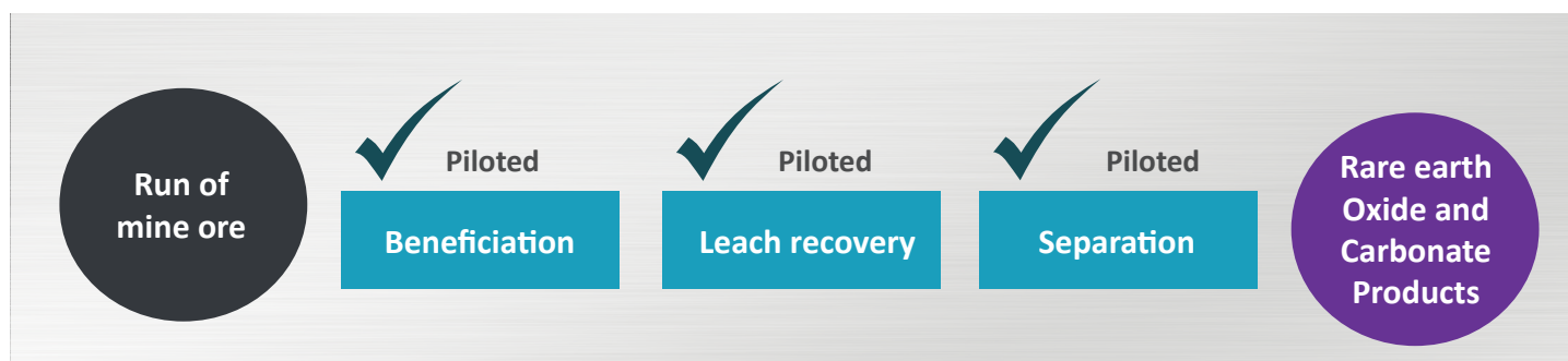
Figure 4: The successful demonstration of the leach recovery and purification pilot plant in October 2016 completed the piloting of the three stage process developed by Peak for Ngualla's rare earth mineralisation.
