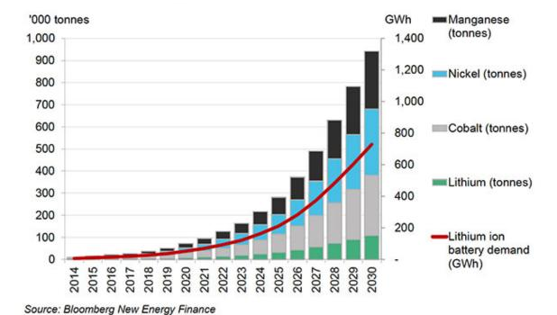
Figure 2: Global lithium-ion battery and materials demand forecast from EV sales, 2015-2030.
