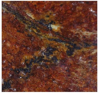
Figure 5: Photomicrograph of polished Mt Thirsty drill core illustrating asbolane veins (black). Image is 4mm across.
