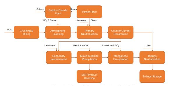
Figure 2: Schematic Process Flowsheet for Mt Thirsty.
