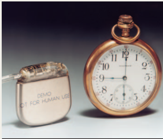
The world smallest pacemaker, a pediatric model powered by a WGT battery.
