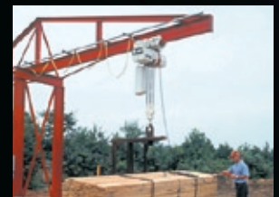
Applications are diverse, including this Coffing electric chain hoist that is lifting and positioning this load of lumber
