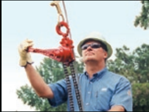
The Company's Little Mule lever tools are widely used by utility linesmen in power distribution
