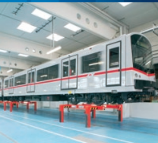
The Metro Vienna, in Austria, uses a Pfaff-silberblau under-floor lifting system with electrically-driven turntables to maintain and repair its trains.
