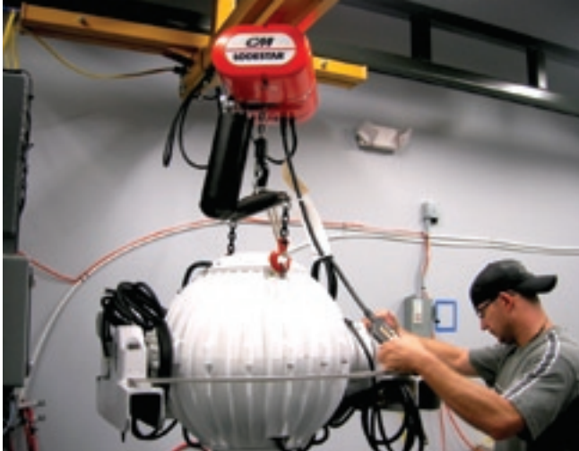
Due to the precise capabilities of the CM Lodestar with Variable Frequency Drive (VFD), a single worker at this Pennsylvania-based manufacturer of stabilizing equipment for ocean vessels can now accurately position a gyro unit for testing.
