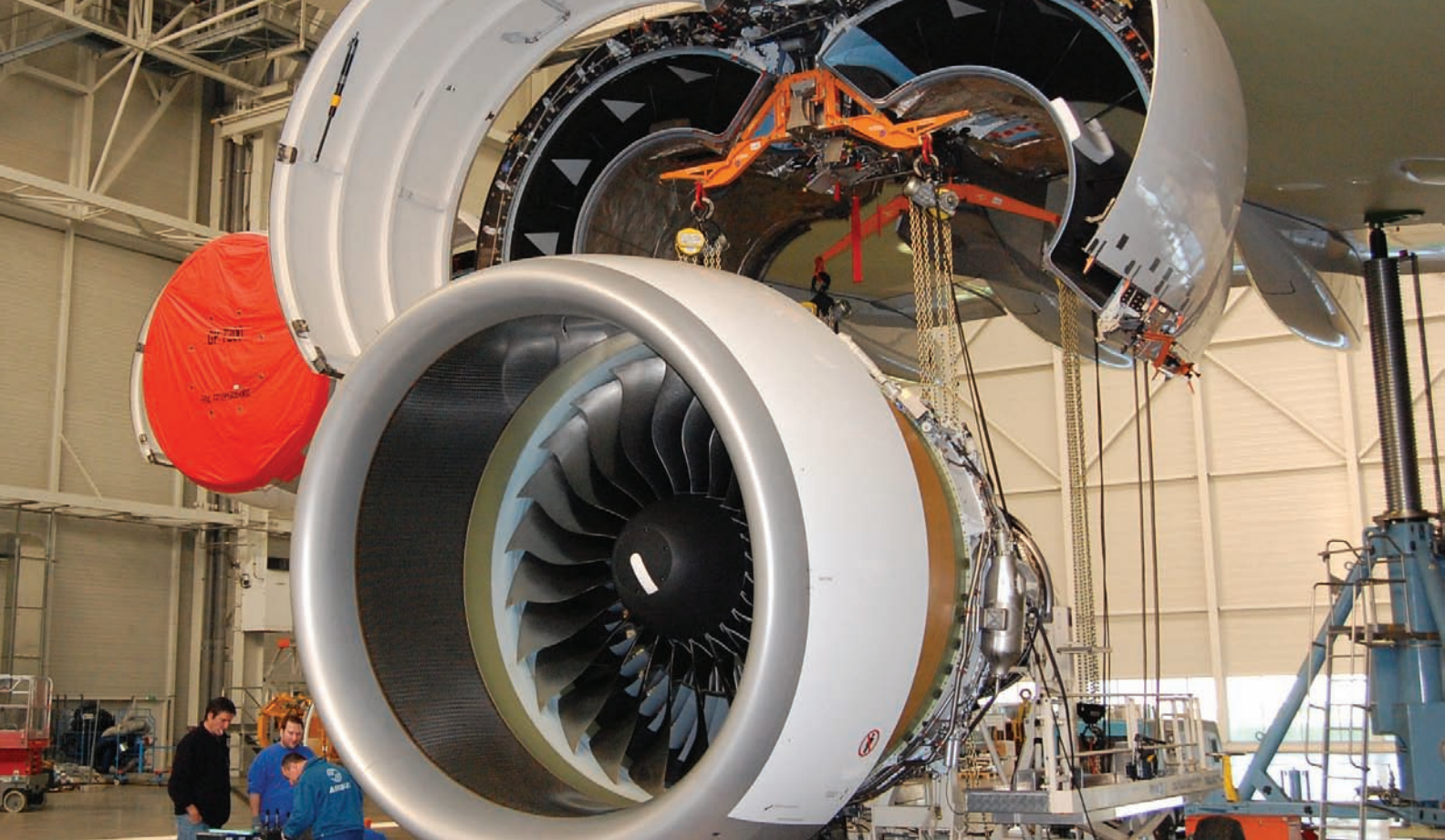
A motorized Yalelift at work servicing an Airbus A380 turbine.
