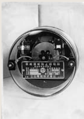
An Early Protective Relay
