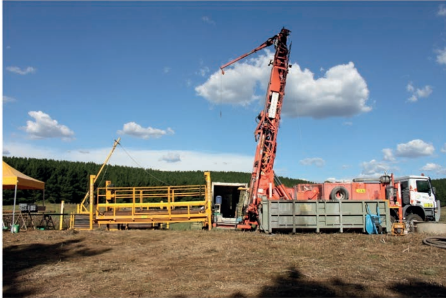
Drill rig operating at the Racecourse project
