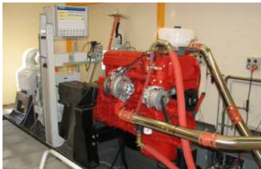
• Orbital's new 600 kW Heavy Duty Engine Test Facility.
