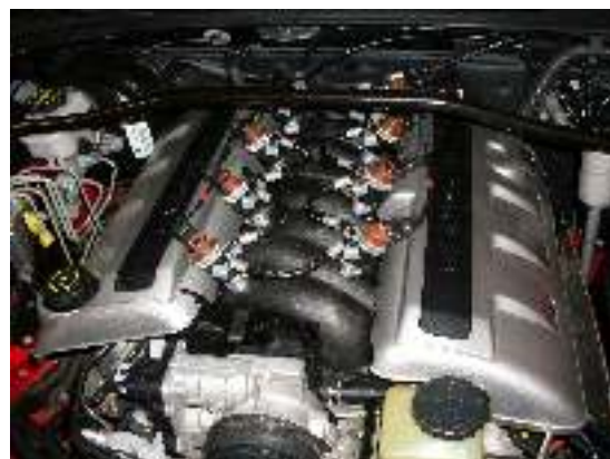
• Orbital Autogas System's Liquid LPG injection systems (LLi) fitted to a V8 automotive engine.
