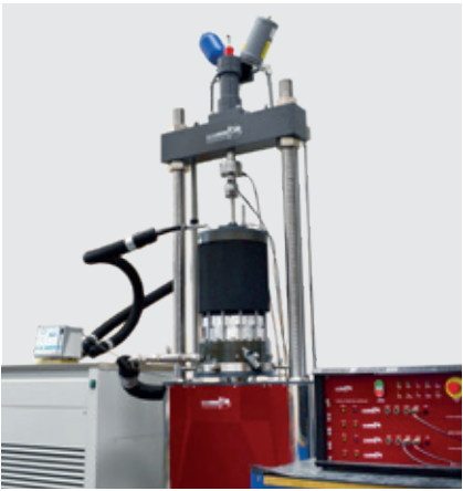
The GDS Hydraulic Loading Frames are load frames with a hydraulic dynamic actuator mounted on the cross beam for axial stress/strain cyclic dynamic loading. This particular frame has our optional temperature controlled heating and cooling system.
