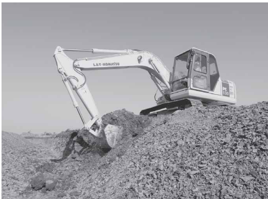
L&T-Komatsu PC130-7 Hydraulic Excavator being employed for canal excavation at an Irrigation project. L&T markets Construction and Mining equipment manufactured within India by L&T-Komatsu Limited as well as machines supplied by Komatsu Limited.
