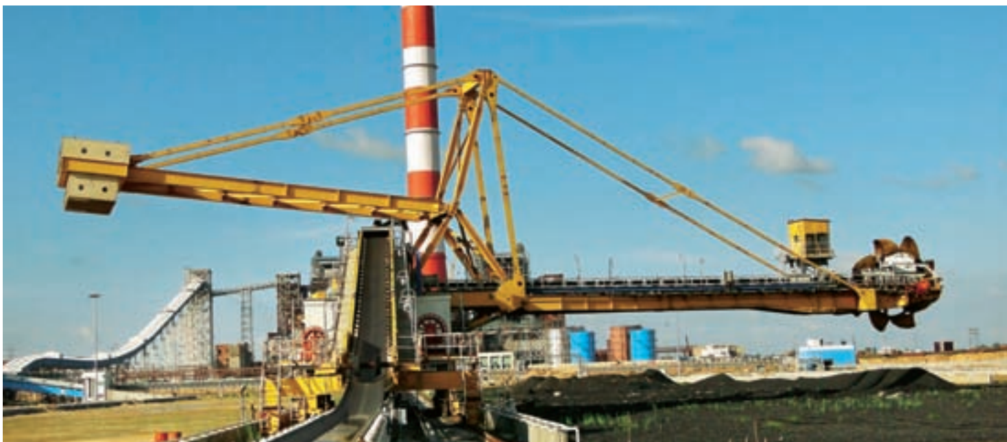
Open stockyard equipped with rail-mounted stacker reclaimers at India's multi-purpose river valley project for Damodar Valley Corporation's Koderama Thermal Power Project in Jharkhand.
