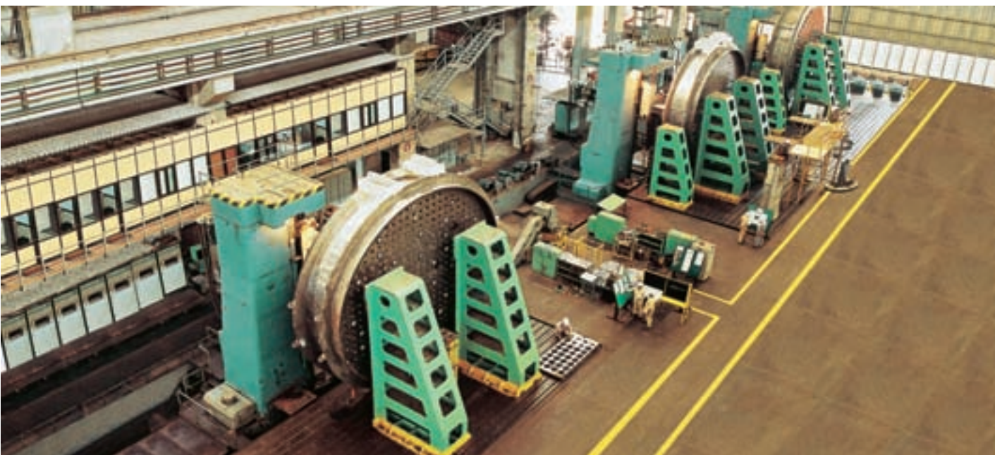
End shields for a nuclear power plant being machined by CNC floor-mounted horizontal boring machines at L&T's Heavy Engineering workshop at Hazira.
