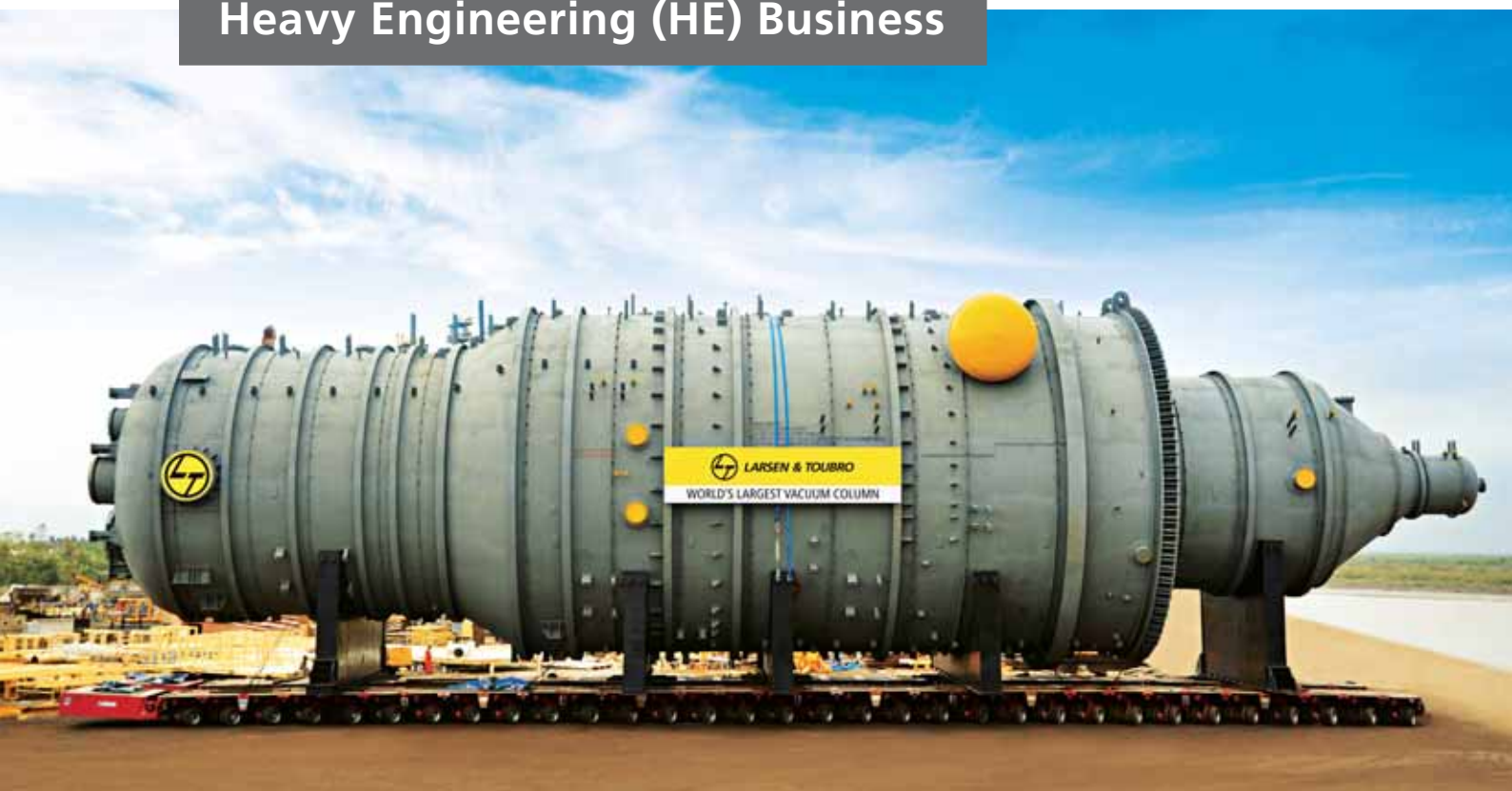
World's largest vacuum distillation column - weighing 975 MT - fabricated by L&T for Paradip refinery (Orissa, India).
