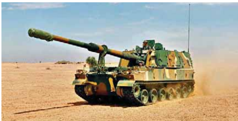
K 9 Vajra T 155/52-calibre self propelled howitzer, designed for all terrains.
