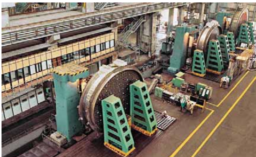
End shields for a nuclear power plant being fabricated at L&T's Hazira facility.
