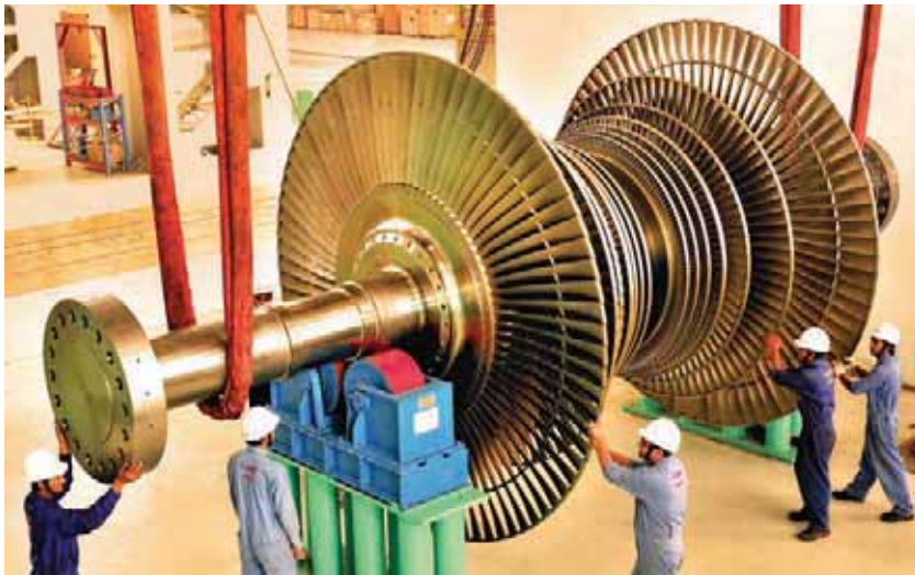
Supercritical turbine being assembled at L&T's Hazira Campus.
