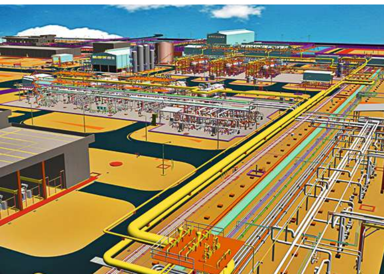
3-D CAD model of Gathering Centre (GC-30) for Kuwait Oil Company
