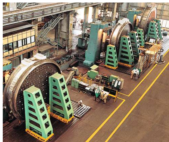
End shields for a nuclear power plant being fabricated at L&T's Hazira facility.
