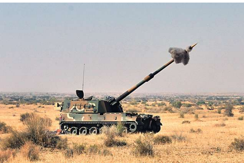
K9 VAJRA-T, a 155mm/ 52 Cal Tracked Self Propelled (SP) Gun, being built in collaboration with Hanwha Techwin.
