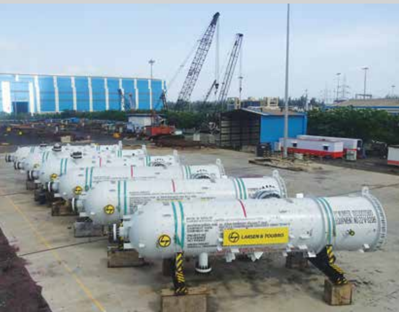
Heavy Thick Vessels (3,312 MT) for KNPC Al-Zour Refinery, Kuwait
