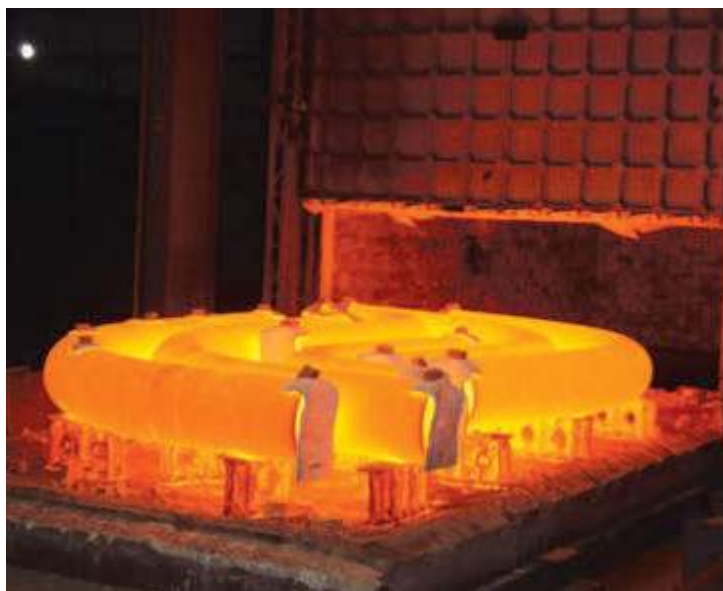
Spools undergoing heat treatment at L&T's forging plant, Hazira
