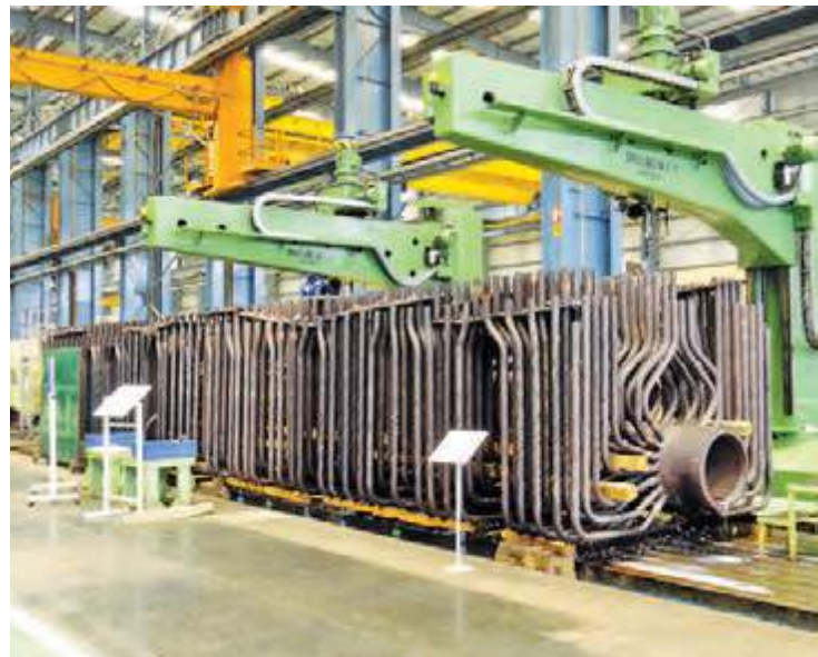
Boiler internals being manufactured at Hazira, Gujarat
