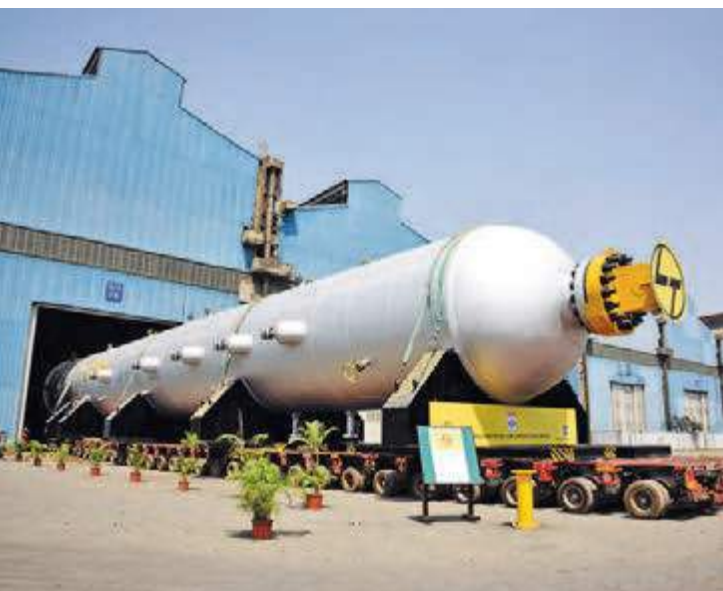
India's heaviest Hydrocracking Reactor (1858 MT) for HPCL Visakh Refinery
