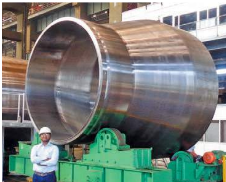
Nuclear Steam Generator Cone Shell - 16 MT
