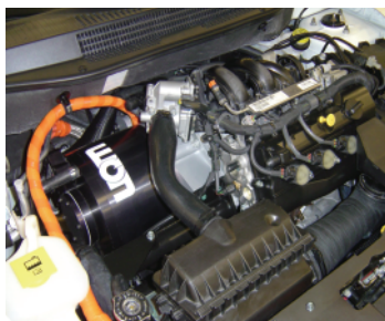
UQM® system under the hood of Caliber ReEV
