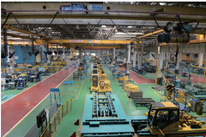
Assembly line for hydraulic excavators at KSC
