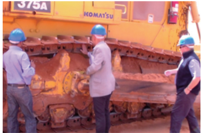
■ Our service mechanics inspecting the wear conditions of D375A's undercarriage
