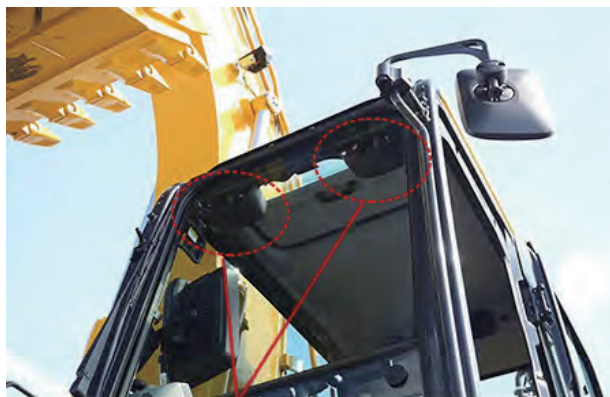
PC200i with a stereo camera (inside the cab)
