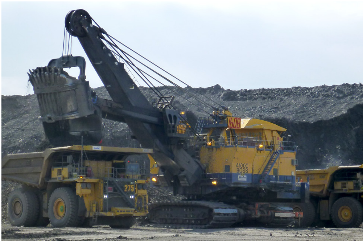
930E AHS dump truck (front and back) teaming up with a 4100C P&H-brand (currently, KMC's brand) electric rope shovel in Suncor Energy's mine in Canada.
