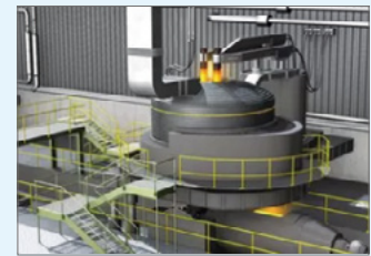
Rendering of next-generation melting furnace using superinsulation
