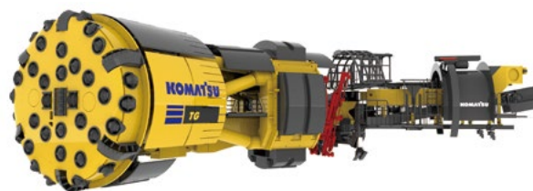
Mining TBM was developed based on the slogan of “No Blasting, No Batch, No Diesel.”
