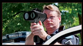
HANDHELD LIDAR SPEED GUN
