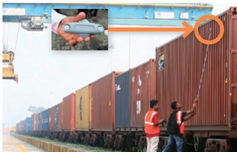
RFID easily attachable to container using magnets
