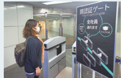
A face recognition access control system that can be used even with masked people (employee gate of NEC Head Office building)
