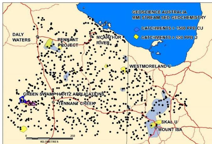
**Figure 9: Geoscience Australia MMI™ stream sediment geochemistry map**
