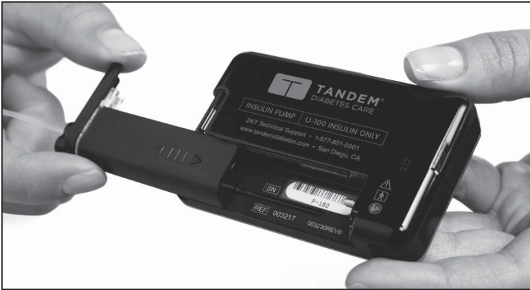
300-unit Insulin Cartridge being inserted into a t:slim X2 pump
