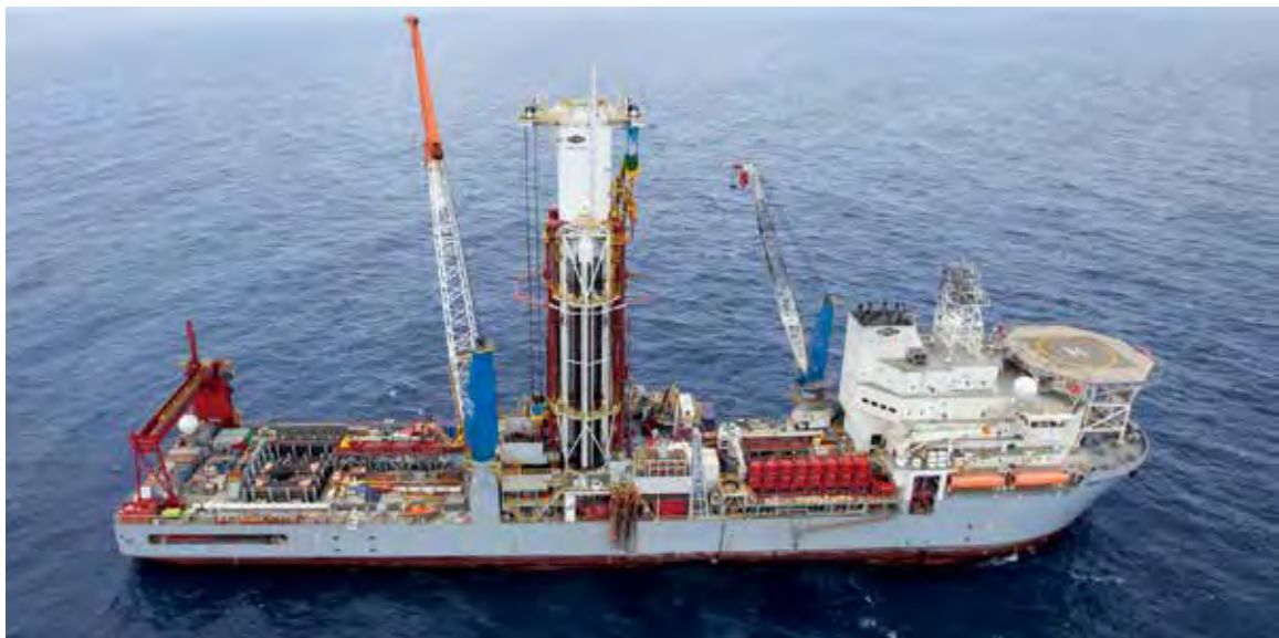
The Noble Globetrotter II has transformed intercontinental mobilisation time and expense for deepwater drilling units. The rig's unique design allows it to transit key gateways between offshore basins, such as the Suez Canal and Bosphorus in a matter of days rather than months.
