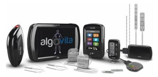
Implantable Pulse Generator: The IPG contains a rechargeable battery and electronics that deliver electrical pulses to the leads. The Algovita IPG has 26 output channels available in two different header configurations and can be connected to one, two or three leads. It is a programmable device and can deliver customized programs for each patient. The IPG is rechargeable and is surgically implanted under the skin, usually above the buttocks or in the abdomen.
