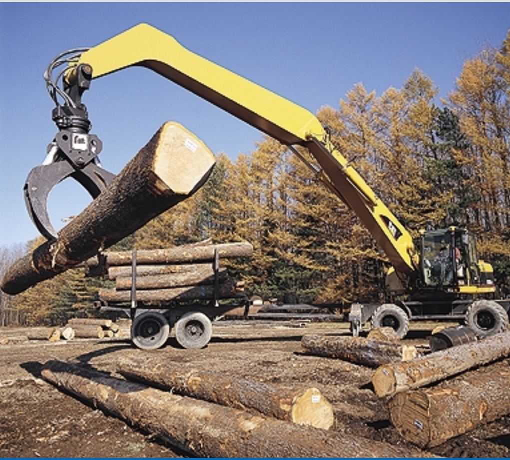
At the sawmill in Marienville, Pa., Highland Forest Resources equipment operator Russ Mainwaring manipulates a cherry veneer log using a Caterpillar 322 log handler. This piece of equipment, purchased in 2003, facilitates the sorting of thousands of logs each year to obtain optimum value.
