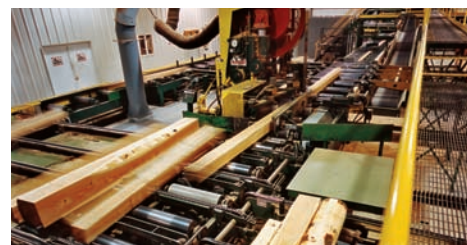
Our Timber segment owns and operates two sawmills in northwestern Pennsylvania. Recent capital investments in these facilities have increased efficiency, not only in their overall operation, but also in their ability to capture and use the waste materials created by the milling process. By-products such as tree bark, wood chips, and even sawdust are sold to and used by a wide variety of local industries.
