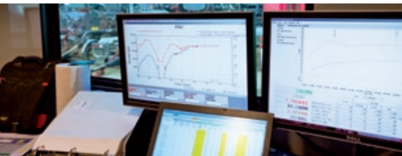
Hydraulic fracturing is a process used to stimulate the flow of natural gas from the rock formations where the gas is located. Here, microseismic monitoring is used to measure the orientation and effectiveness of a hydraulic fracture in one of Seneca's Marcellus wells.
