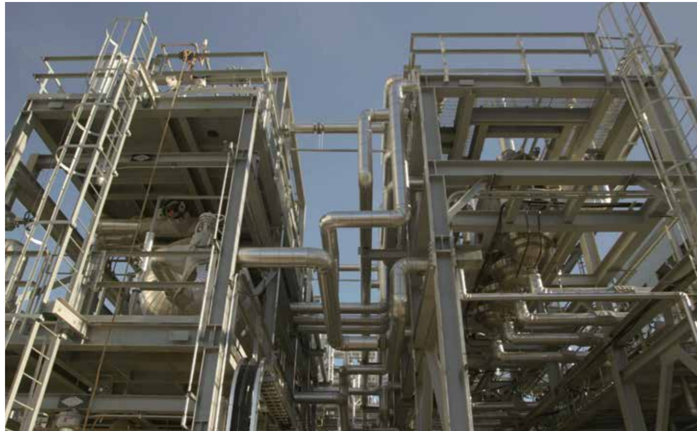
Some of the Fischer-Tropsch modules including those incorporating the Velocys Fischer-Tropsch reactors (right).
