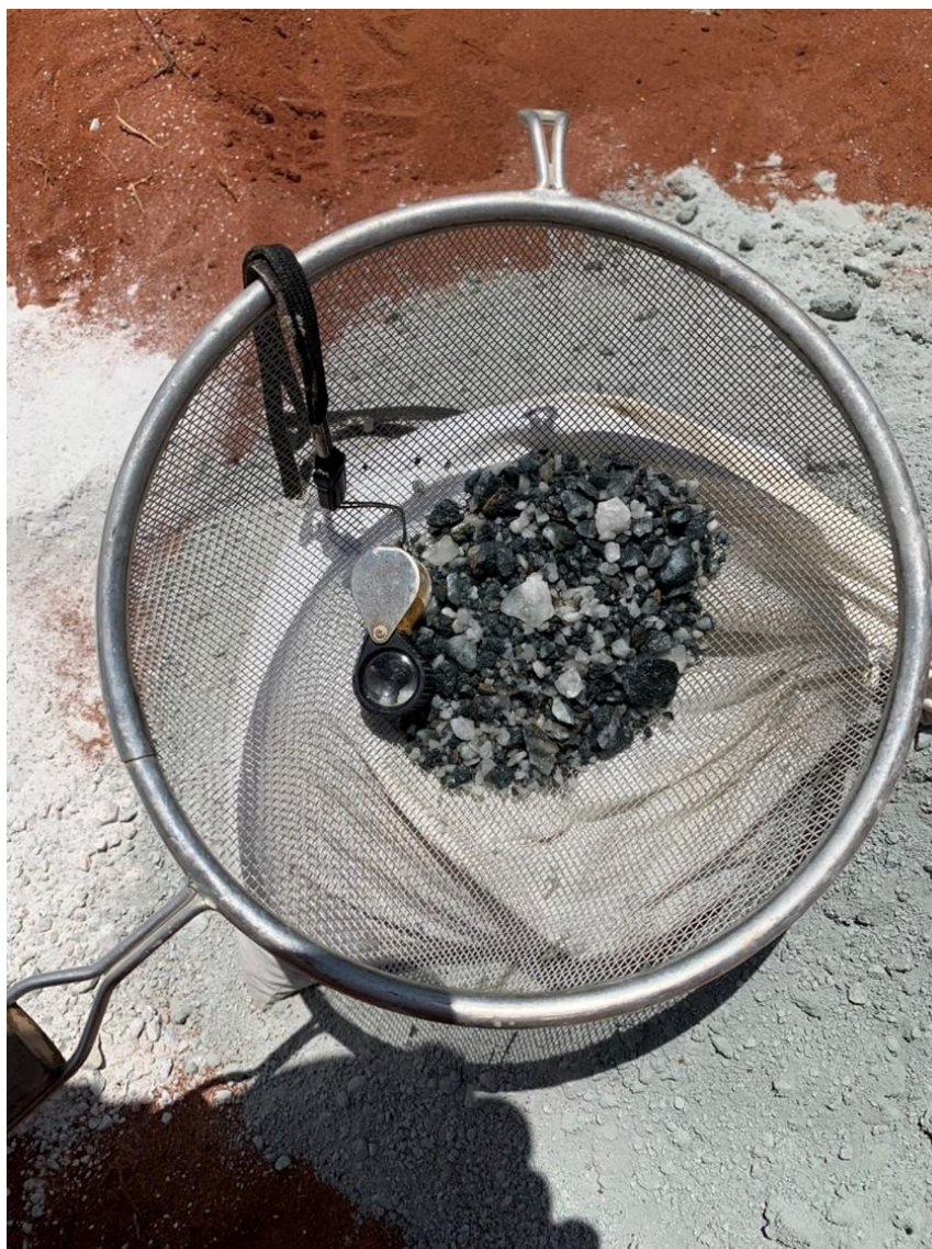
Photo 6: 21BRC0012 - Quartz carbonate veined mafic-ultramafic intrusive showing 3-5% disseminated sulphide (pyrite).
