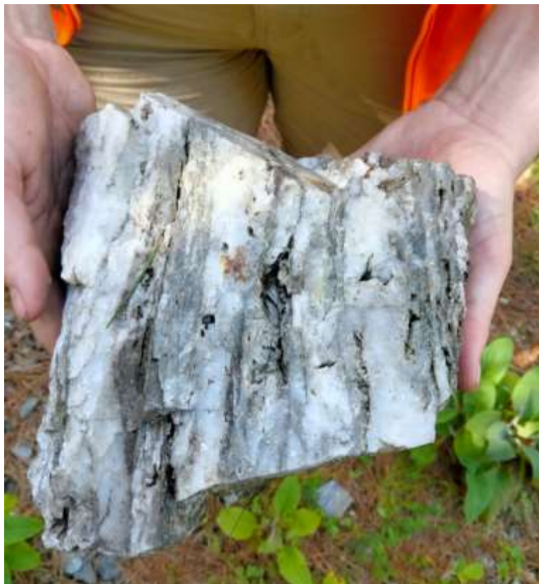
Figure 9: Weathered Golden Bar Quartz vein showing ribbon banded quartz textures with defuse wall rock inclusions and some stylolitic planes. This vein texture is typical of high-grade mesothermal orogenic gold deposits
