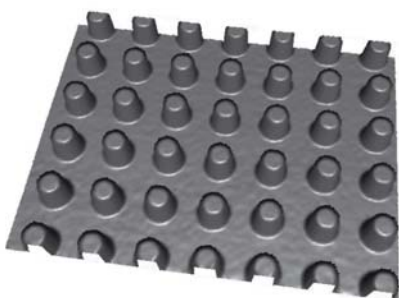
An example of micro-fabrication using “Nanoimprint” technology
