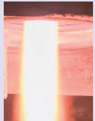
Plasma in an in-flight melting furnace
