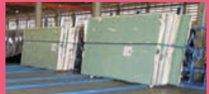
Leaning storage of large flat glass
